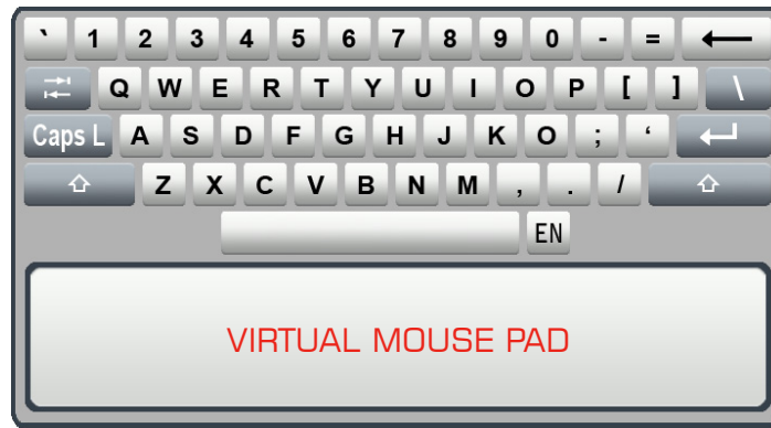
Fig. 2 The Virtual Keyboard (VK) and Mouse Pad allow protecting against both keystroke and mouse logging. The users can either click directly with the PC mouse pointer on the VK's buttons or operate the virtual mouse pointer before selecting which button to click.
